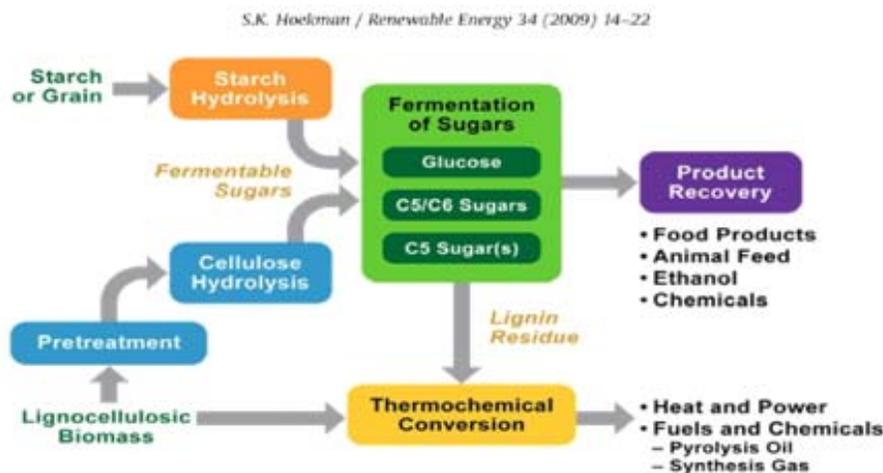
Figure 6. Bioethanol processing from maize grain and biomass (Hoekman 2009).
